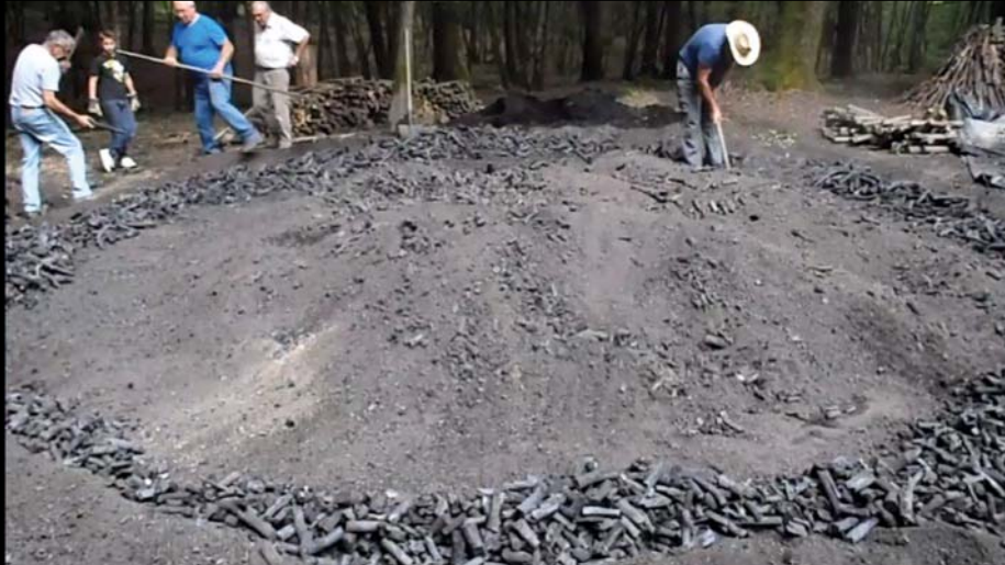
Extraction of charcoals from the middle to the outside during the unloading of the kiln (photo Aurore Dupin)
